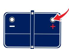
Connect the positive terminal, first and check the terminal clamps for tight fit, when installing new battery.
