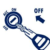
Switch off the engine and keep sparks, flames, cigarettes away from battery at all times, before removing the old battery.
