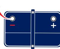
Disconnect the negative terminal, first and avoid short-circuit caused by tools, when removing old battery.
