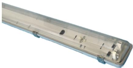
This compact IP65 batten design, is a durable and robust, made of polycarbonate base and diffuser, powder coated steel gear tray and G13 lamp holders. Clear diffuser makes it ideal for T8 LED tubes. Suitable for domestic, Industrial and commercial installations.
